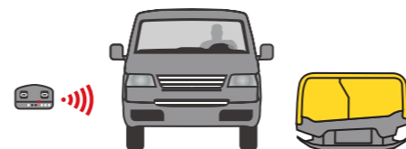
High level of safety: It stops moving automatically if there is no clear line of sight between the operator and the compaction equipment.
