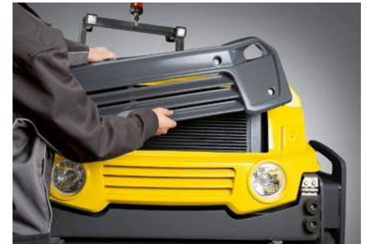
Easy radiator cleaning due to separately removable flap.
