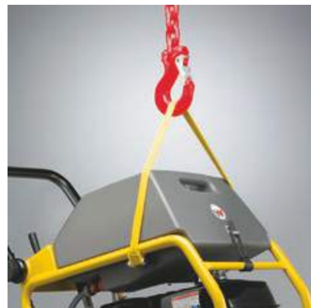
The central lifting point provides balance and ensures that the rear wheels always touch the ground first.
