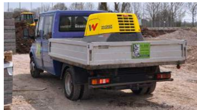
A low loader is not necessary: The DPU130r only weighs 1,200 kg and can be transported on a truck bed.
