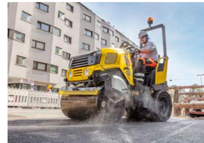
Tapered design: for an unobstructed view of the drum edges, the machine surroundings and the construction site.
