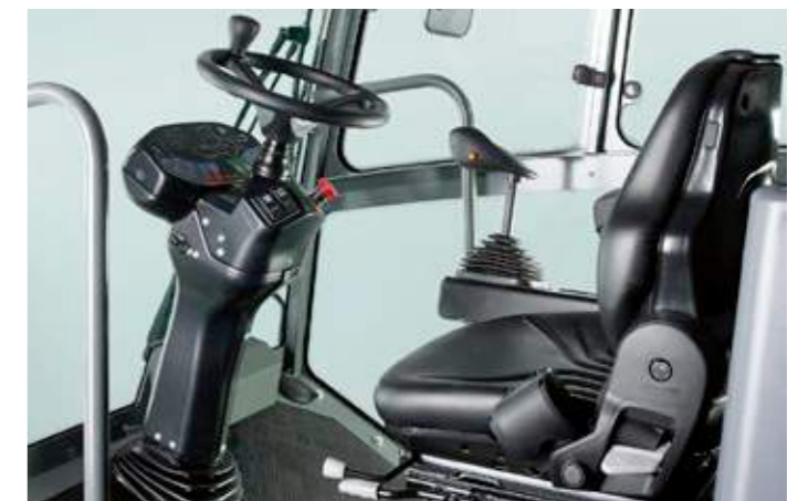
Comfort for the operator: The seat and steering column can be individually adjusted.
